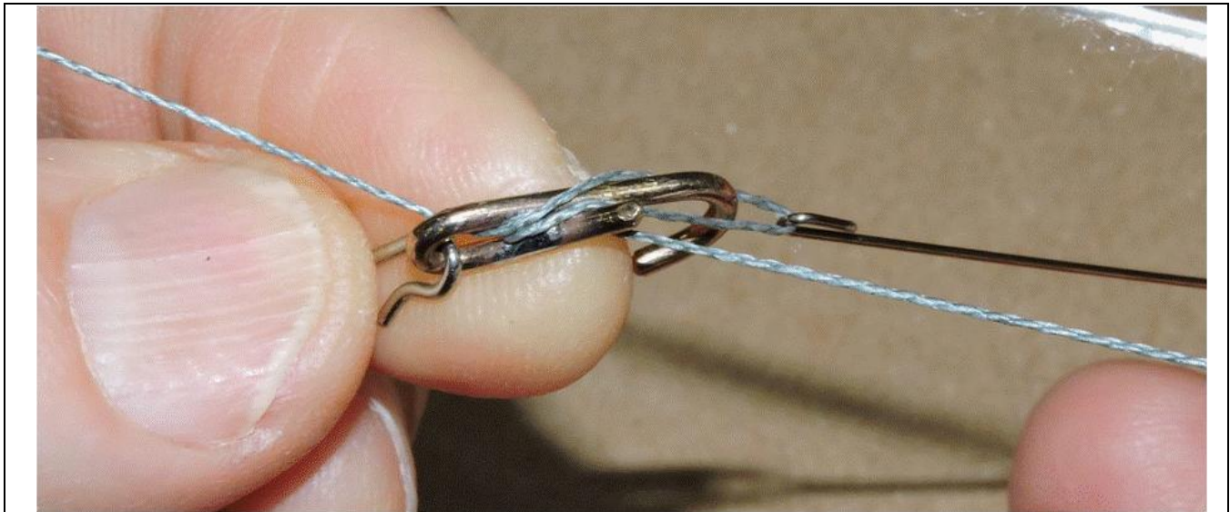
Figure 5. Hook Installation on the Haulage Rope
