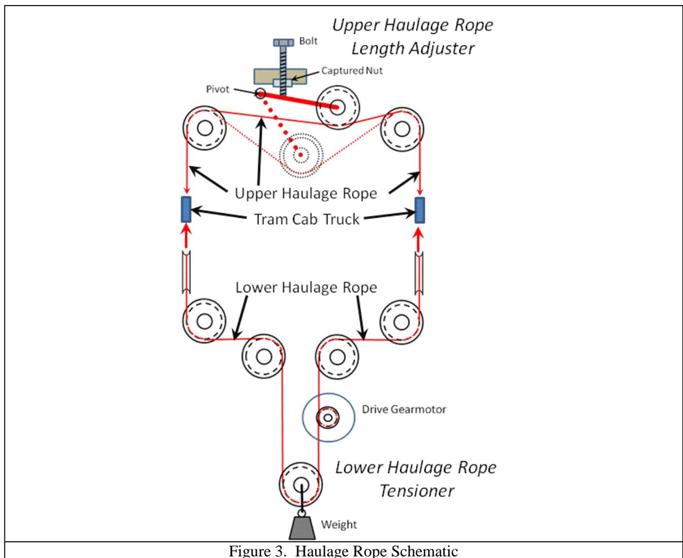
Figure 3. Haulage Rope Schematic
