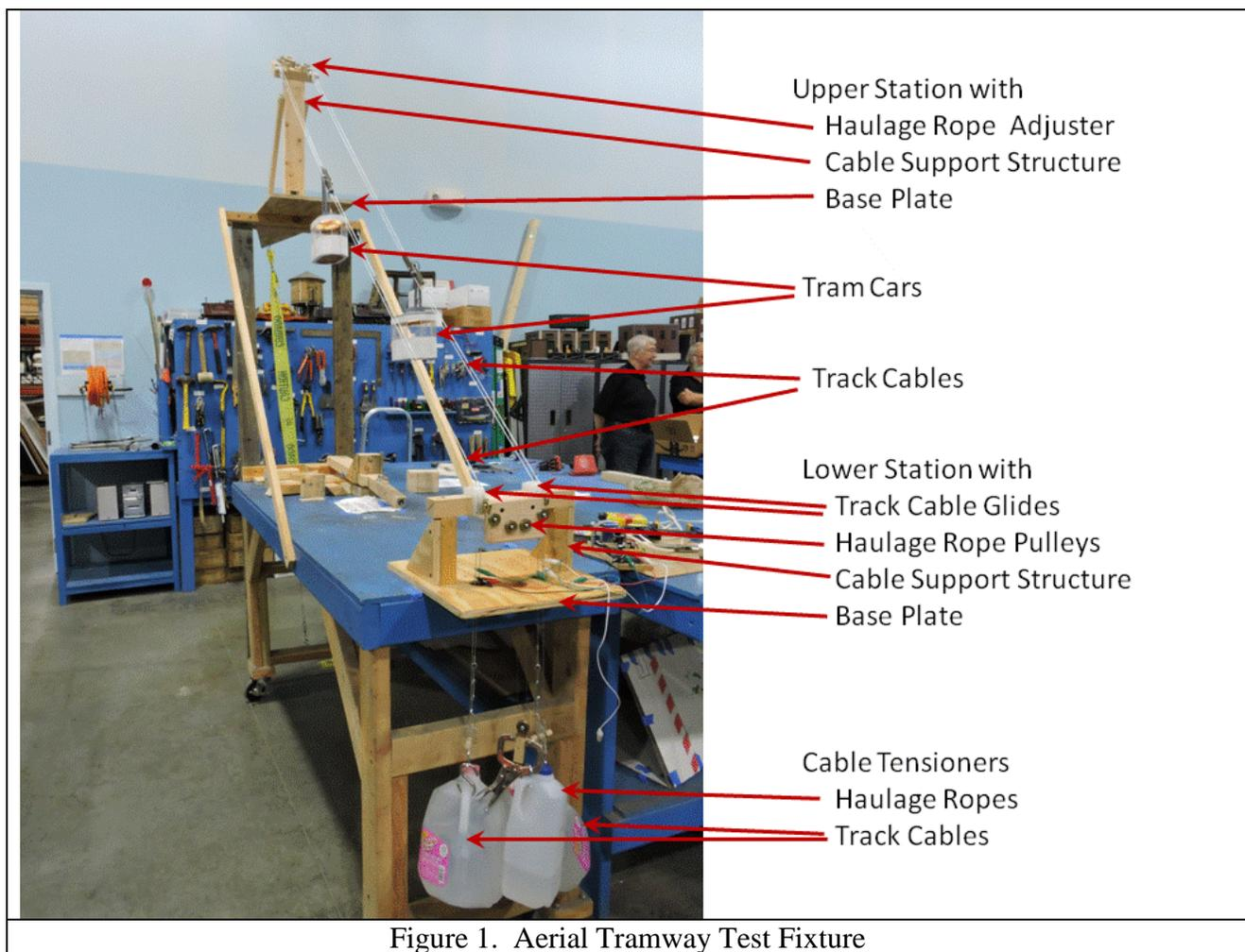
Figure 1. Aerial Tramway Test Fixture
