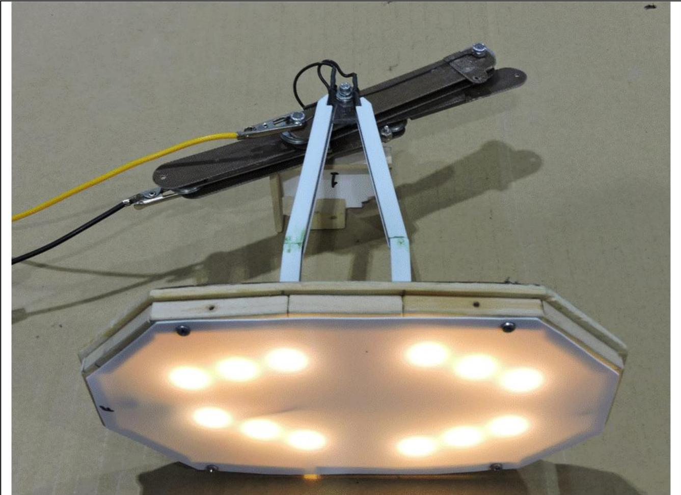
Figure 5. Tram Cabin Lighting Diffuser
