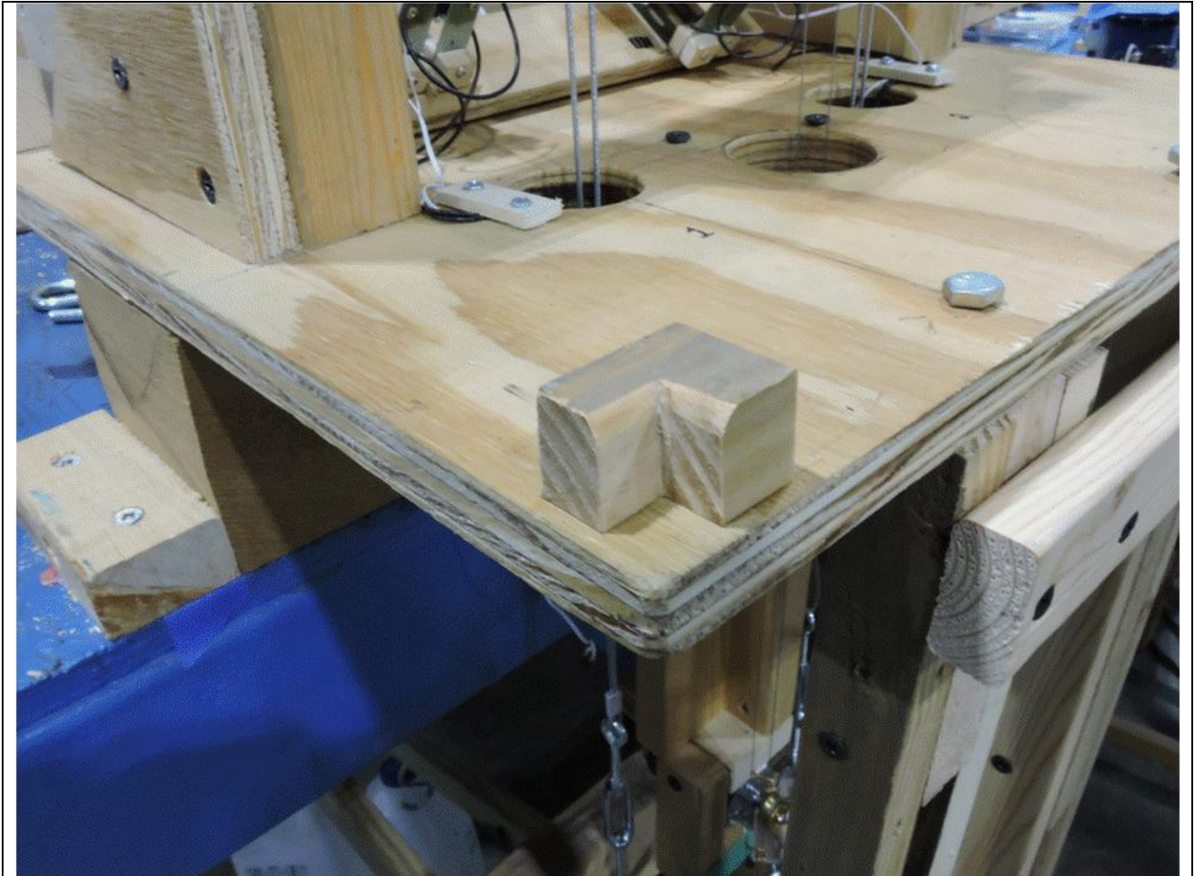
Figure 4. Station Building Locating Block
