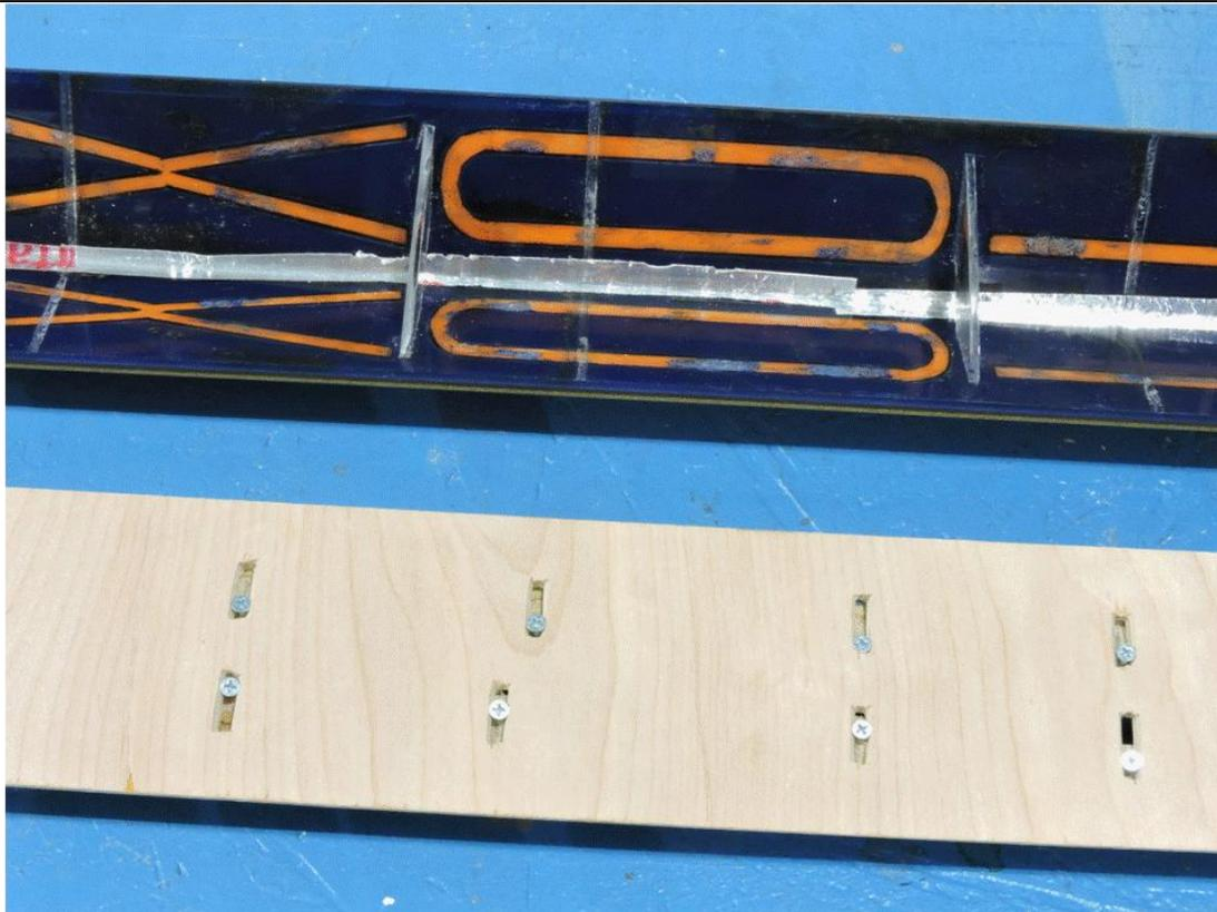
Figure 4. Light Position Adjustment Detail
