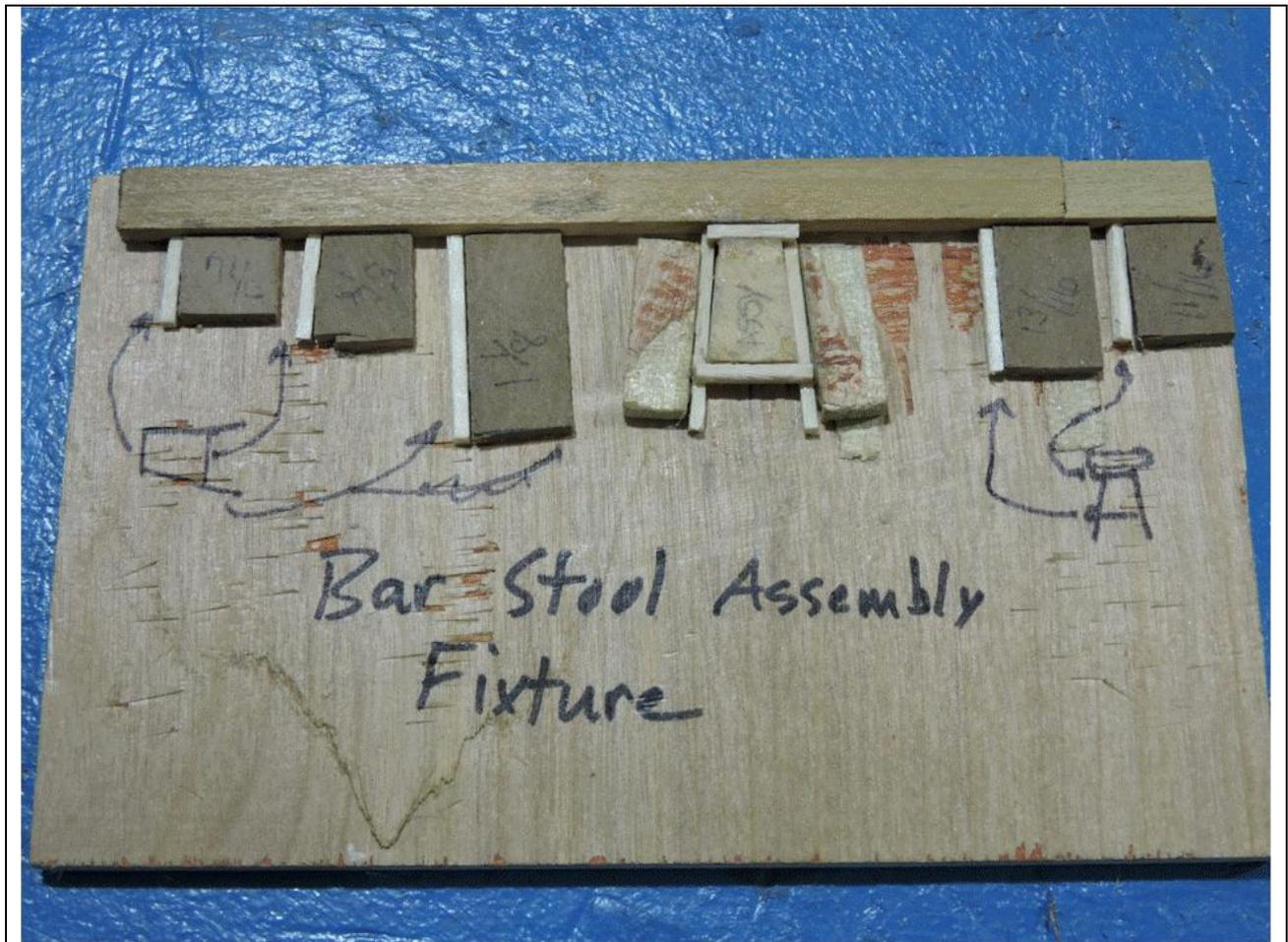
Figure 3. The Cutting and Two-Leg Set Assembly Fixture
