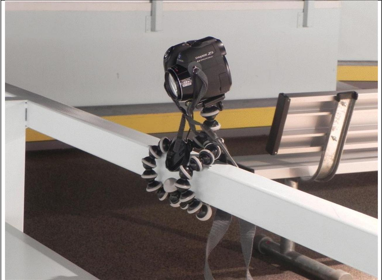
Figure 4. Gorillapod in Conventional Mounting
